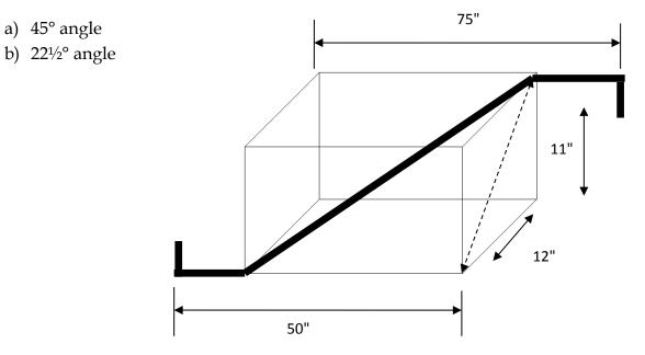
Task 2: Calculate the setback and diagonal for the following pipe schematic using a
