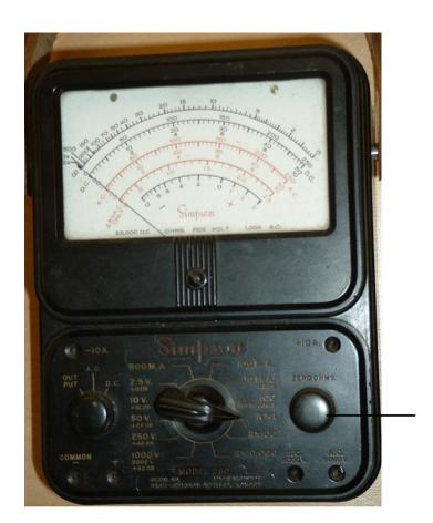
c) The ohmmeter should display some value if the stove element is working
