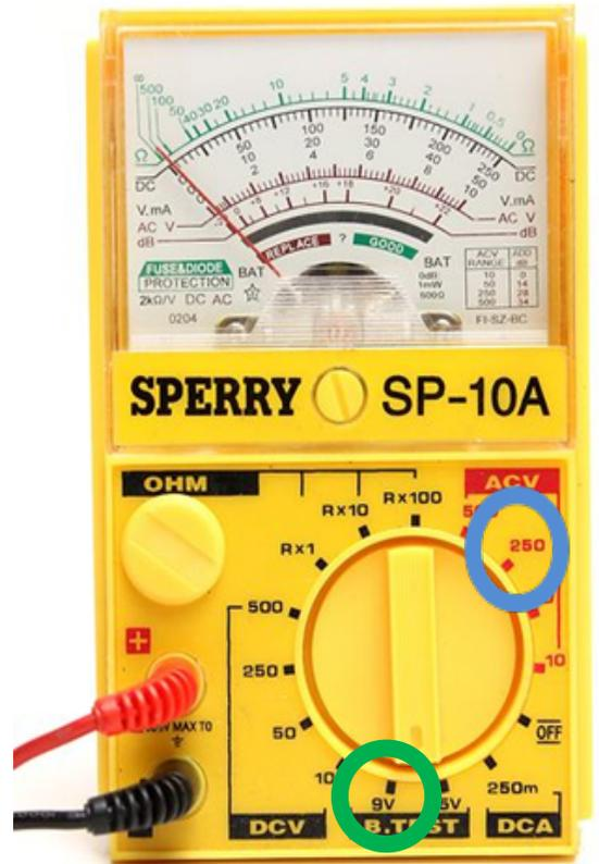
**Task 1d: Batteries are considered in working order at 70% voltage or better. A 9 Volt battery reading shows the needle at about 43%. In what range will the needle point?**
