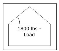
Step One - Determine the angle of the sling
